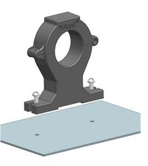
Base Plate Screw M4 (gasket) Installation
